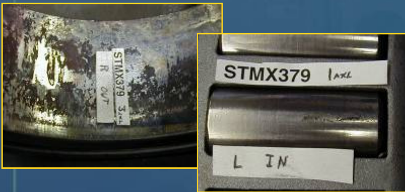
Loose cone with roller spalling, detected by large cup spall
