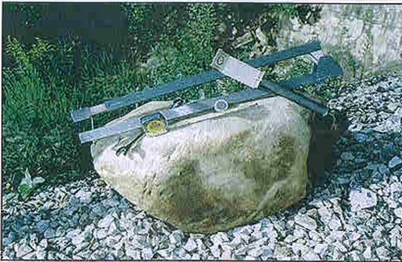
Figure 5-9: Servo alignment fixture, adjustable wrenches, and tape line
