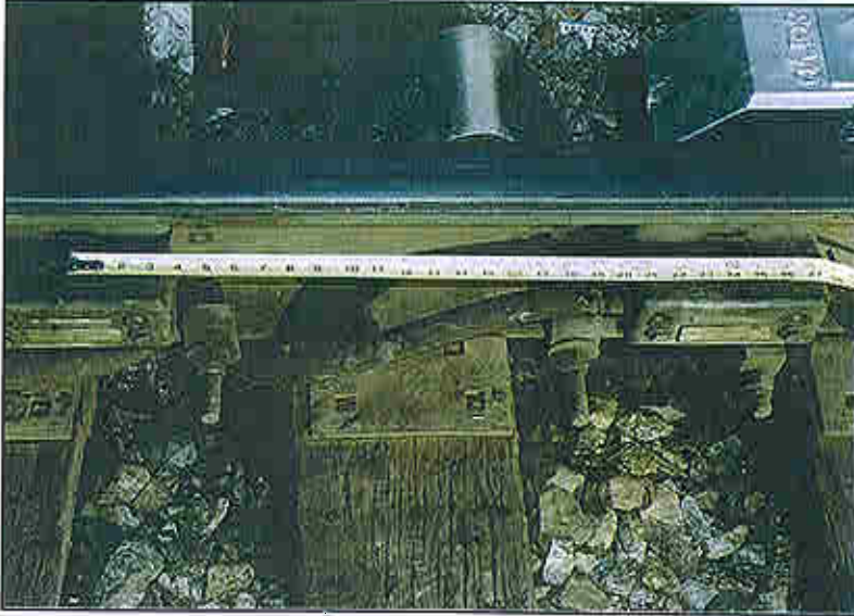
Figure 5-16: 24 inches between the A and B transducers
