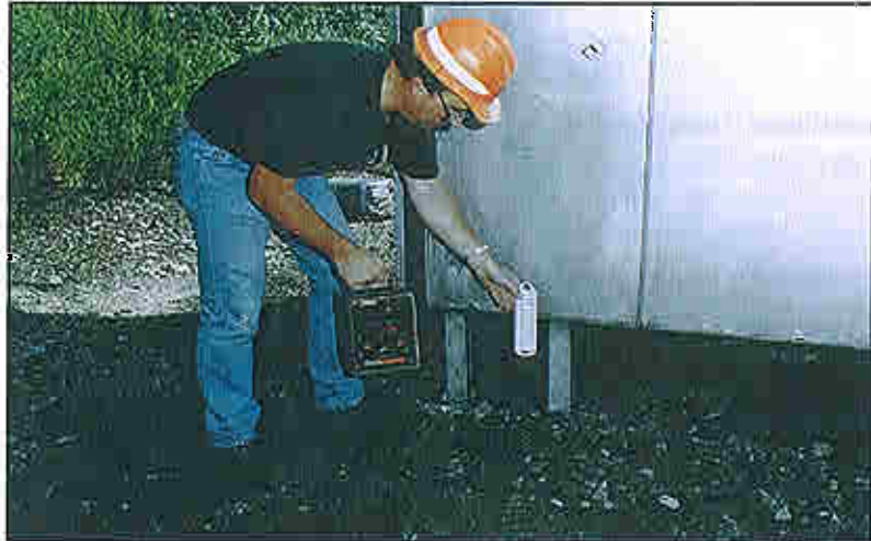
Figure 5-7: Placing the function simulator/generator in the shade
