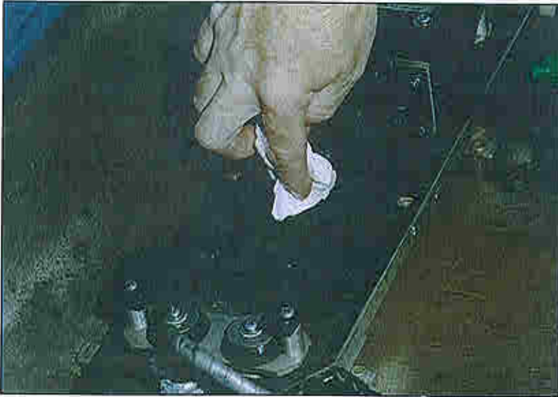
Figure 5-4: Cleaning the scanner lenses
